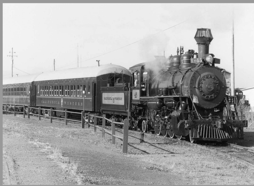
California Western RR tourist train ready to depart from Fort Bragg, California, Locomotive #45, a Baldwin built Mikado (2-8-2) was built in 1924. This shot was taken during Wallace's post convention trip down the Oregon-California coast. photo by Wallace
